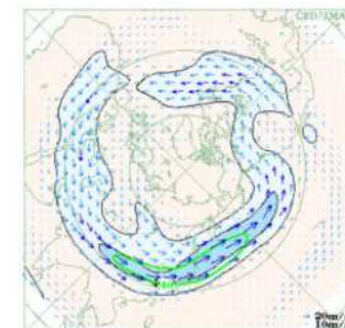
Fig. 5 Monthly mean 200-hPa wind speed and vectors in the Northern Hemisphere (October 2010). Black lines show wind speeds at an interval of 20 m/s. Blue shading shows values greater than 40 m/s. Green lines show normal wind speeds at an interval of 40 m/s. Base period for the normal is 1979-2004.
